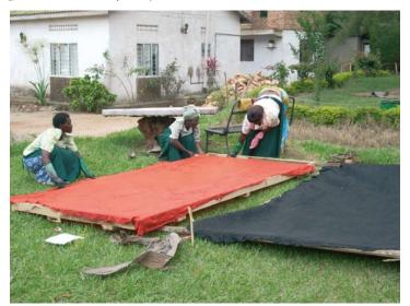
9. The finished cloth is stretched out on a frame. It is then laminated on a non-woven backing in order to create a high-quality wallcovering.
